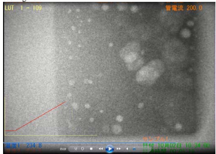
Figure 7. Large Voids Photographed as Solder Reaches Liquidus
