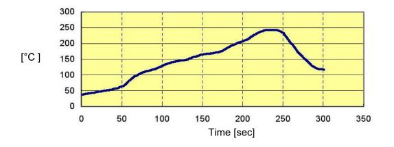
Example of Reflow Temperature Profile- 5 Zones, Hot Air Reflow Furnace
