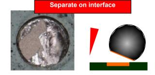
Shear starts from the solder not from the joint interface. The joint strength provided by this solder paste is sufficient.
