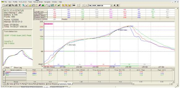
Note: Profiles using a soak time > 60 seconds may require nitrogen for satisfactory results Use of air for long soak profiles has resulted in dull, grainy joints, and possible de-wetting of solder joints.
