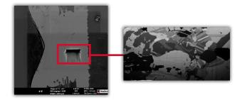
The low-stress Via Dep 4550 enables thermomechanical benefits compared to regular electroless copper processes and can provide optimal grain structure at the via interface.
