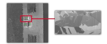
Compared to standard electroless copper plating, the via interface with Blackhole direct metallization is simpler and has fewer areas for reliability concern, while also allowing for environmental benefits.
