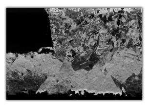
Via Dep 4550 provides the optimal grain structure at the target pad interface for reliable microvias.
