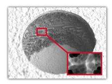
Direct plating allows for a single interface of electrolytic copper to the microvia target pad, eliminating the need for flash plate and electroless copper and reducing the number of potential separation points. The low-etch direct metallization processes **Blackhole LE** and **Eclipse LE** are especially well suited to the challenges of mSAP for SL-PCB and IC substrate designs.
