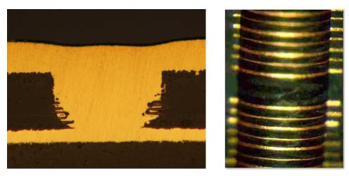
**Blackhole** enables a uniform electrolytic plating and an intimate copper-to-copper bond for the highest reliability interconnects.
