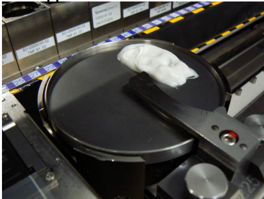
Flux Dispensed in Rotating Application Tray
